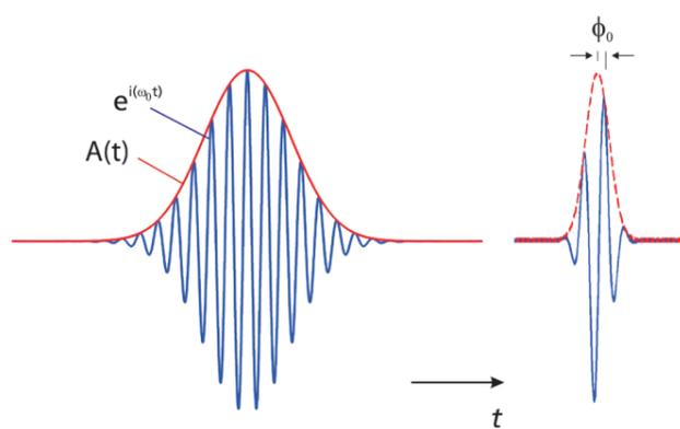
Figure 1: A comparison of two femtosecond pulses with the corresponding electric field oscillations. In the few-cycles pulse shown, the Ti:sapphire centre frequency of 375 THz, a wavelength of 800 nm respectively, the period of the electric field oscillation is 2.7 fs.
