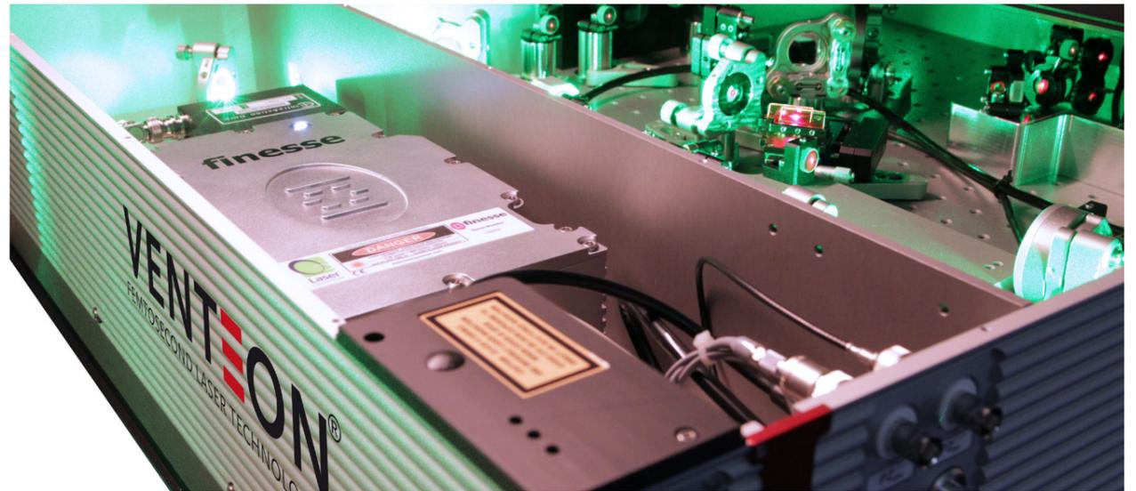
Figure 2: An image of the Finesse 6 Pure (Laser Quantum Ltd) pumping an octave-spanning VENTEON | PULSE : ONE femtosecond oscillator
