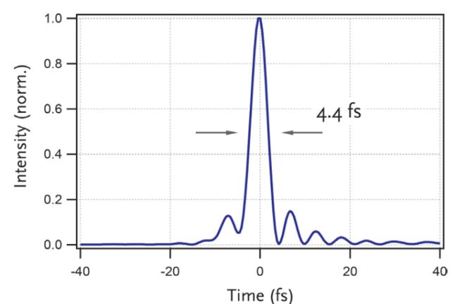
Figure 3: A SPIDER characterised pulse of 4.4 fs is shown: the shortest commercially available pulse from a CEP-stabilised Ti:sapphire laser.
